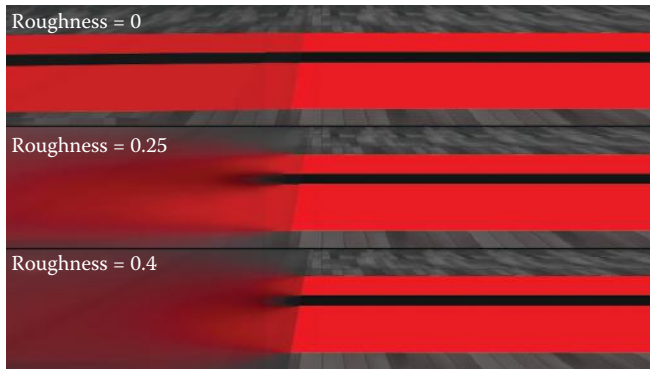
Figure 4.28. Another example of Hi-Z Screen-Space Cone Tracing producing spread reflections the farther it travels due to micro fracture simulation using material roughness.
